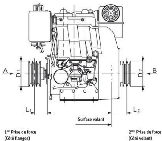
$$D_1 \text{ (mm)} \geq 700 [45+L_1 \text{ (mm)}] \quad \frac{N \text{ (kW)}}{n \text{ (RPM)}}$$
